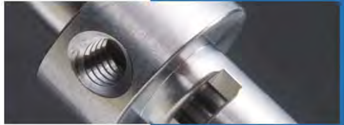
Implantable pacing component – Stainless steel turned and threaded on Swiss turning center; EDM produces slot.
