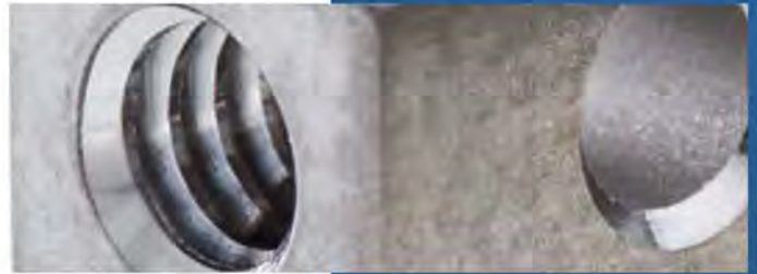
Pacing connector block – Dedicated manufacturing cell with 9-axis Swiss turning center and 5-axis wire EDM.
